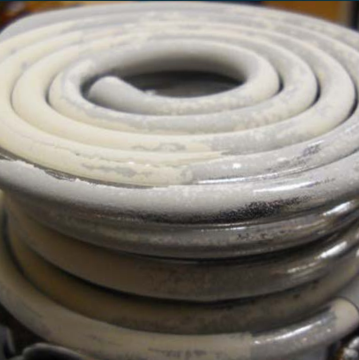
ELECTRICALLY INDUCED PRECIPITATION
